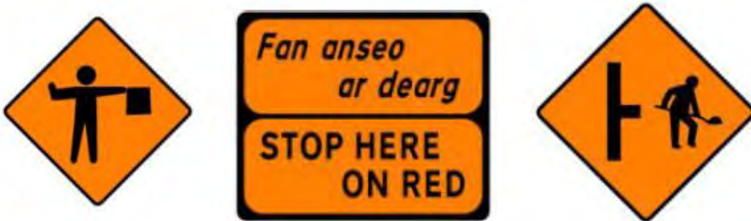
Figure 7 – Sample Road Signage
